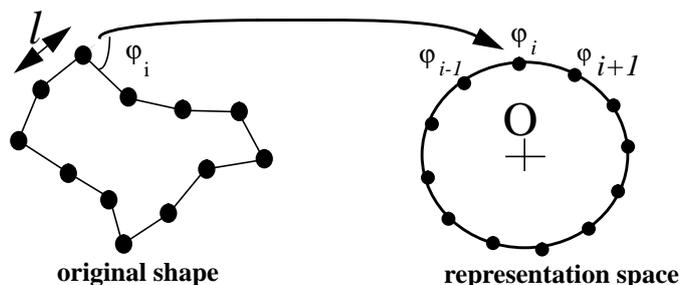
Figure 4: Mapping between shape and circular representation space.
