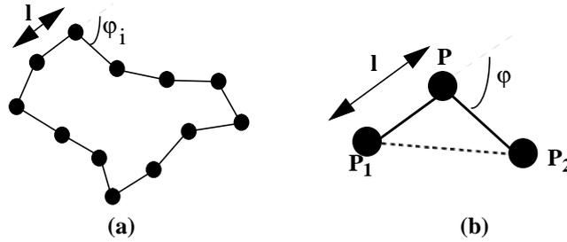
Figure 2: Discrete curvature measure of a 2-D curve.
