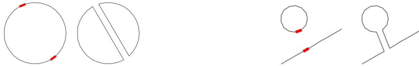
Fig. 3. Topological operator applying on (left) two edges on the same connected component or (right) two different connected components.
