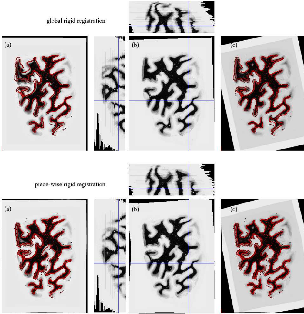
Fig. 9. Reconstruction of a 3-D histological volume with a globally rigid (top) and our piece-wise rigid (bottom) registration algorithm: (b) coronal view (middle) of the 3-D reconstructed volume corresponding to the 51 st image of the stack with the associated axial (top) and sagittal (left) views, (a) 50 th image (immediately preceding section) with edges of the 51 st one superimposed in red, (c) 52 nd image (immediately following section) with edges of the 51 st image superimposed
