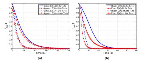
**Fig. 2.** (a) Mappings  $t \to F_{T_d(app)}(t)$  and  $t \to F_{T_d(sim)}(t)$  for two different hyper-exponential distributions (N = 10). (b) Comparison of CCDF of  $T_d$  in the case of hyper-exponential (simulated CCDF) and exponential (CCDF using (16)) inter-meeting time distributions (N = 50).
