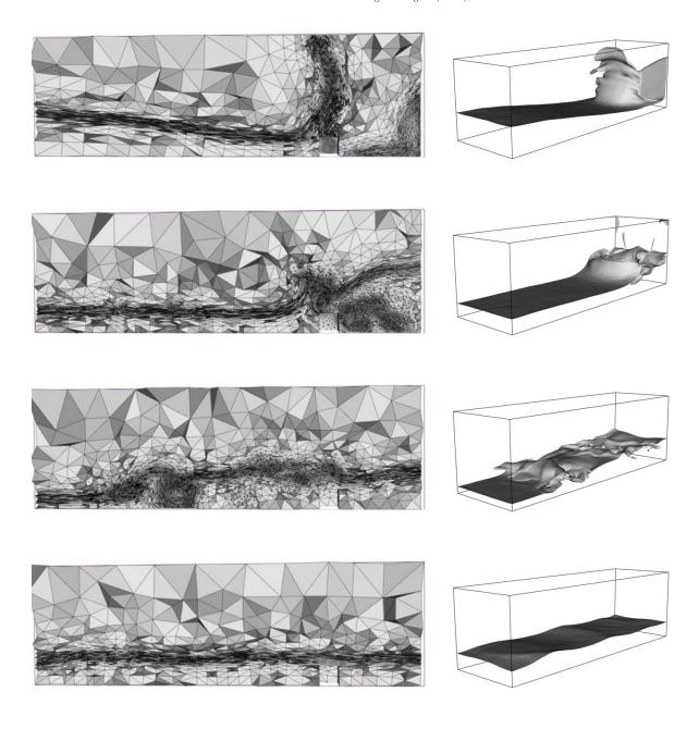
Fig. 10. Dam break simulation: cuts in the volume meshes for times 0.85s, 1s50, 2.50s, and 7s50 (left) and representation of the interface water/air (right).
