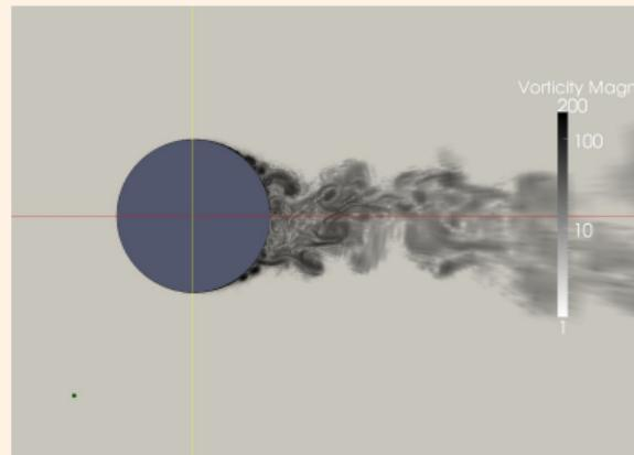
Circular cylinder (1.2M nodes), iso-contours of the vorticity magnitude.
