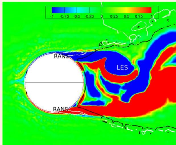
Instantaneous isocontours of spanwise vorticity (simulation GR1-LRS). The lines are the isolines of the blending function:  $\theta = 0.1$  (black) and  $\theta = 0.9$  (white)
