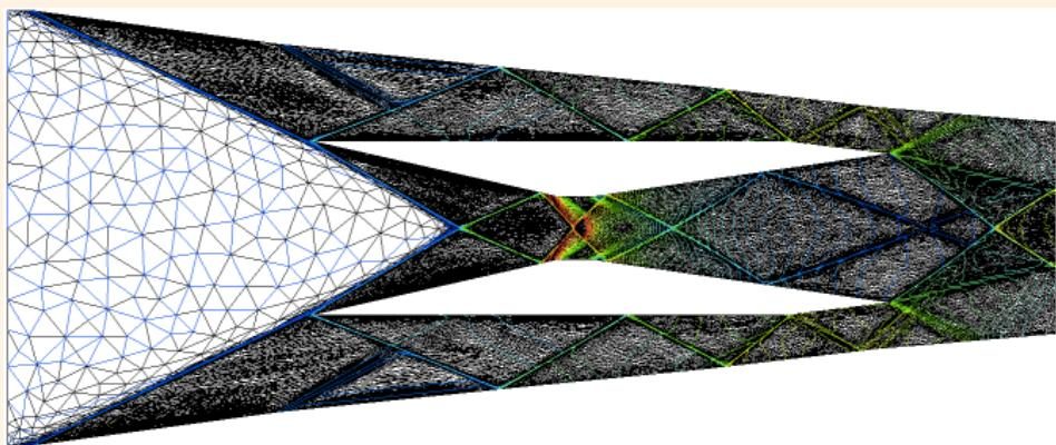
**Figure:** 2D anisotropic mesh adaption (31460 nodes), iso-contours of Mach number. Inlet Mach number = 3, CENO scheme.
