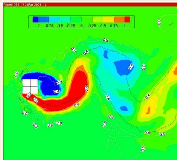
Isocontours of spanwise vorticity. The lines are the isolines of the blending function:  $\theta = 0.4$  (black) and  $\theta = 0.9$  (white).
