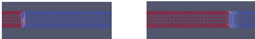
Figure 2: Zooms on the moving contact discontinuity using a load balancing procedure at two different time steps
