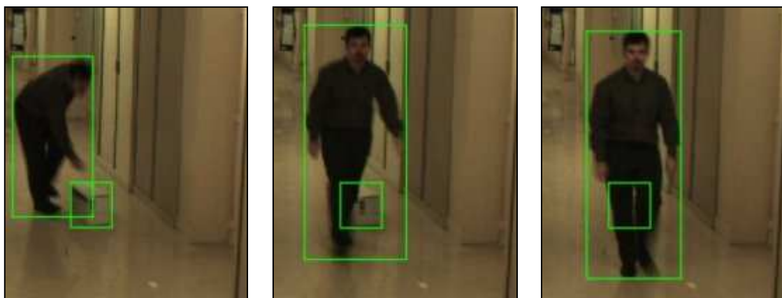
Image 5. Example of dynamic occlusion annotation: (a) the box is not occluded (b) the box is partially occluded (c) the box is completely occluded.
