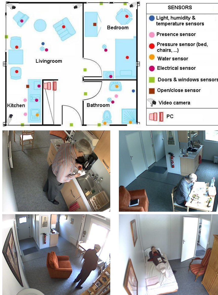
Figure 1: Homecare monitoring: the set of sensors embedded in an apartment and the different views of the apartment captured by 4 video cameras
