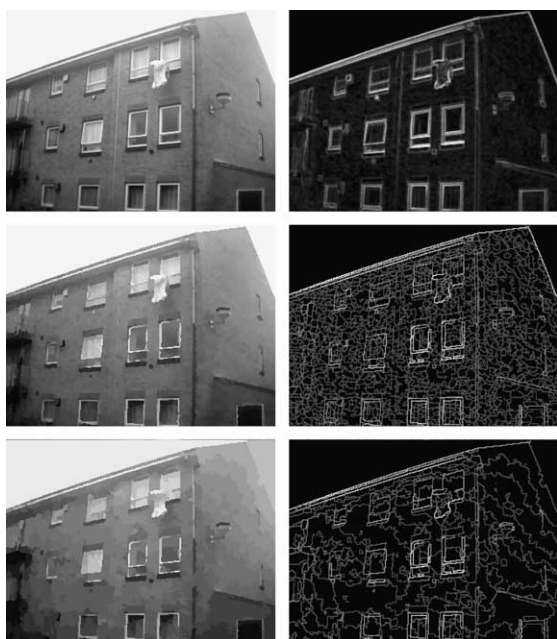
Fig. 5. Results obtained for the ‘House’ image. Top row: original and gradient images; middle row: mosaic and weighted watershed images after using the watershed algorithm; bottom row: simplified mosaic and weighted watershed images after using the proposed algorithm.
