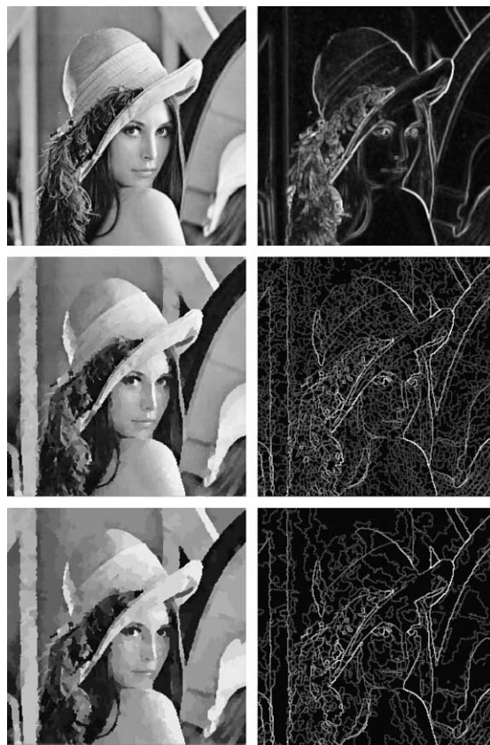
Fig. 6. Results obtained for the ‘Lena’ image. Top row: original and gradient images; middle row: mosaic and weighted watershed images after using the watershed algorithm; bottom row: simplified mosaic and weighted watershed images after using the proposed algorithm.
