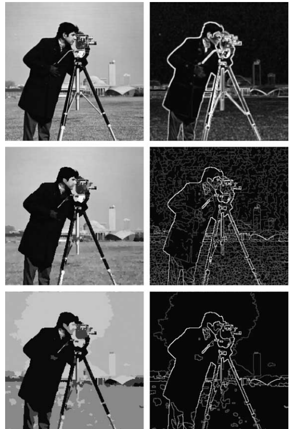
Fig. 4. Results obtained for the 'Cameraman' image. Top row: original and gradient images; middle row: mosaic and weighted watershed images after using the watershed algorithm; bottom row: simplified mosaic and weighted watershed images after using the proposed algorithm.
