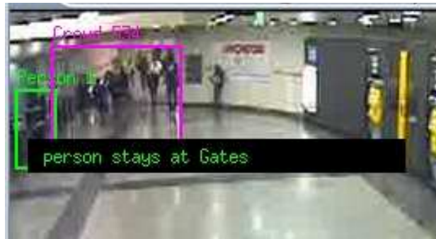
FIG. 4 – A person with label '1' and a crowd with label '534' are tracked. The event 'person' stays at gates has been detected.
