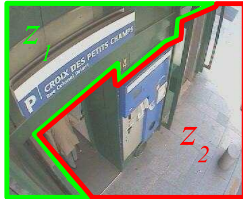
Figure 7.1: Example of a local tuning based on a priori knowledge of the scene. The tuning of the detection thresholds for pixels in z_1 should be less sensitive to variations than for z_2 .
