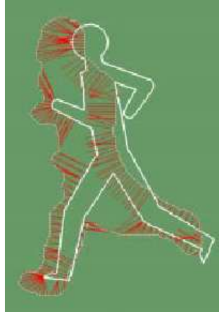
Figure 2.10: Continuous white lines are the contour of the silhouette of the projected 3D model. Dotted white lines are those of the real silhouette. Red lines are the forces necessary to match the contours [Delamarre and Faugeras, 2001].
