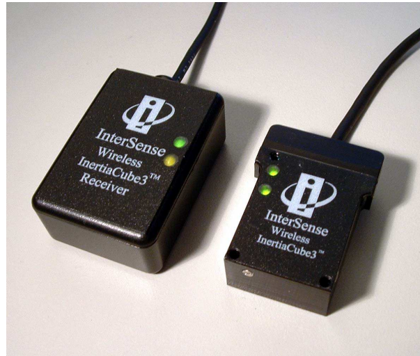
Figure 2.2: Wireless inertiaCube 3: the receiver and the marker [Intersense, 2006].
