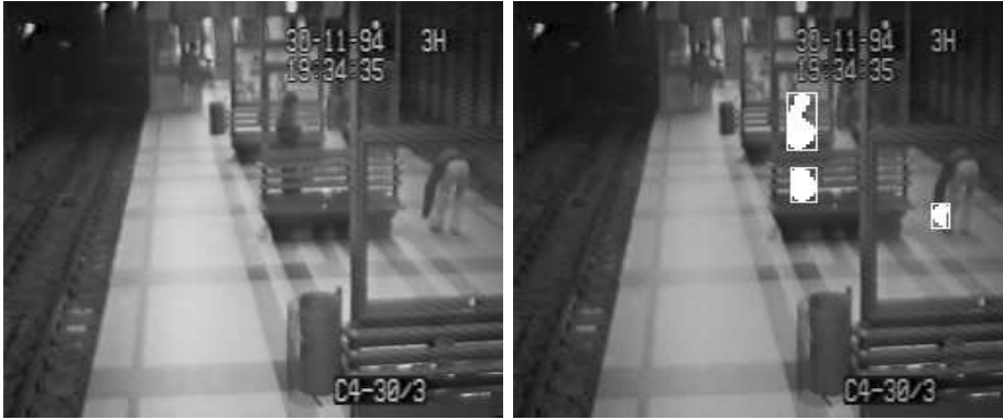
Figure 2: Frame 1 is a raw image taken from the image sequence. Frame 2 is the result of the moving region detection task. It shows two moving regions partially occluded by the back of a seat.
