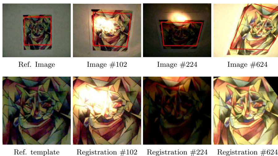
Figure 4.8. (Top) Direct image registration of a reference image to successive color frames of a video sequence. The sequence contains severe changes in the specular, diffuse and ambient reflections. (Bottom) Registered images demonstrate the stability of the alignment.
