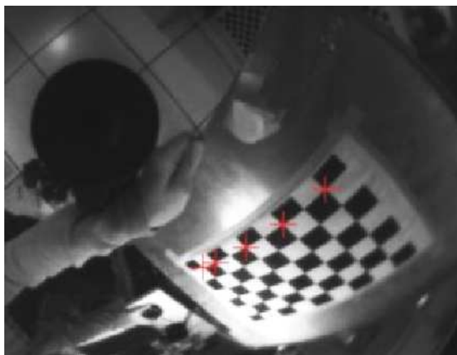
Figure 3.2: Estimation of the generalised focal length from line image points
