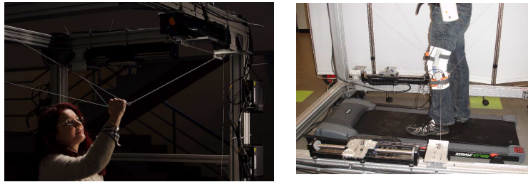
Fig. 2 MARIONET-REHAB used in rehabilitation tasks. The wires and the 3D accelerometers will be used to precisely measure human joint motion during a rehabilitation task.
