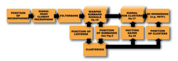
Figure 6.9 Overview of the synthesis algorithm used to re-render the acquired soundscape based on the previously obtained subband positions.
