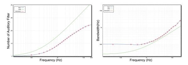
**Figure 2.3** Comparison between BARK and ERB scale. The right plot shows the bandwidth as a function of the central frequency. The left plot shows the number of auditory filters up to each frequency value.
