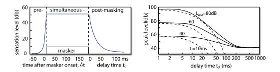
Figure 2.5 Temporal masking : (a) Regions where premasking, simultaneous masking and postmasking occur. (b) Peak level of a  $20-\mu$ s Gaussian pressure impulse as a function of the delay time after the offset of white noise maskers of a given level [Zwicker and Fastl, 1999].
