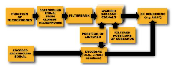
Figure 7.2 Overview of our re-synthesis pipeline. Foreground sound events are rendered as point sources while background sounds are encoded using a low-order spherical harmonics decomposition.
