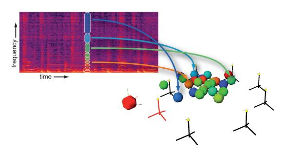
Figure 6.8 In the resynthesis phase, the frequency components of the signal captured by the microphone closest to the location of the virtual listener (shown in red) is warped according to the spatial mapping pre-computed in the off-line stage.
