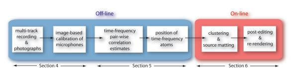
Figure 6.1 Overview of our pipeline. In an off-line phase, we first analyze multi-track recordings of a real-world environment to extract the location of various frequency subcomponents through time. At run-time, we aggregate these estimates into a target number of clustered sound sources for which we reconstruct a corresponding signal. These sources can then be freely postedited and re-rendered.
