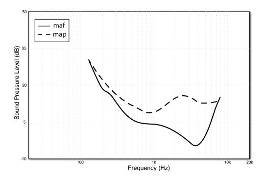
**Figure 2.7** Minimum sound level as a function of the frequency [Moore, 1997]. The solid curve show the minimum audible pressure at the eardrum (MAP). The dashed curve show the minimum audible pressure in a free sound field (MAF).
