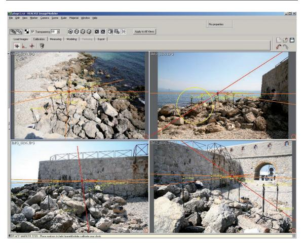
Figure 6.2 We retrieve the position of the microphones from several photographs of the setup using a commercial image-based modeling tool. In this picture, we show four views of a recording setup, position of the markers and the triangulation process yielding the locations of the microphone capsules.
