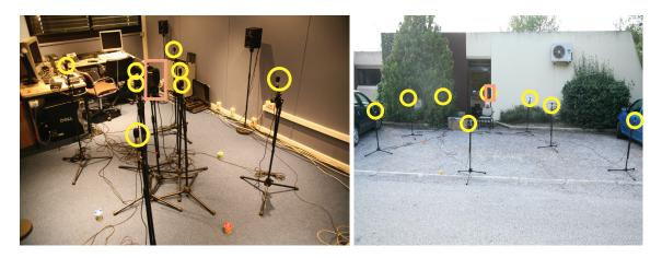
Figure 7.4 Example recording setups. We used 8 omnidirectional microphones (circled in yellow) to capture the auditory scene as well as a *Soundfield* microphone (highlighted with a light red square) to simultaneously record a B-format version. A binaural recording using microphones placed in the ears of a subject provided a reference recording in each test case.
