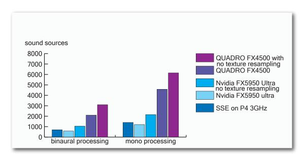
Figure 4.5 Performance tests for audio rendering on the CPU and GPU.
