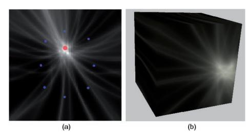
Figure 6.5 (a) A 2D probability histogram for source location obtained by sampling a weighted sum of hyperbolas corresponding to the time-difference of arrival to all microphone pairs (shown in blue). We pick the maximum value (in red) in the histogram as the location of the frequency band at each frame. (b) A cut through a 3D histogram of the same situation obtained by sampling hyperboloid surfaces on a 3D grid.
