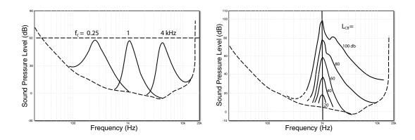
**Figure 2.4** Simultaneous masking : (a) Level of test tone just masked by critical-band noise with level of 60 dB, and center frequencies of 0.25, 1 and 4 kHz. The broken curve is the threshold in quiet. (b) Level of test tone just masked by critical-band white noise with center frequency of 1kHz and different levels as a function of the frequency of the test tone [Zwicker and Fast], 1999].
