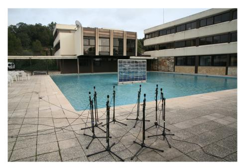
Figure 6.13 Microphone setup used to record the fountain example. In this case the microphones are placed at the center of the action.
