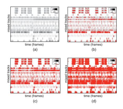
**Figure 5.3** (a) Loudness values (using Zwicker's loudness model) through time for the 17 tracks of a musical mix. Each track was selectively filtered and processed into 4 frequency sub-bands resulting in 68 signals to prioritize. (b) Priority map showing the first 12.5% most important frames highlighted in red. (c) First 25% most important frames and (d) first 50% most important frames.
