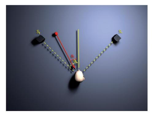
Figure 3.6 Stereophonic law of sines. A phantom source (red sphere) is created using an intensity panning between the two speakers.
