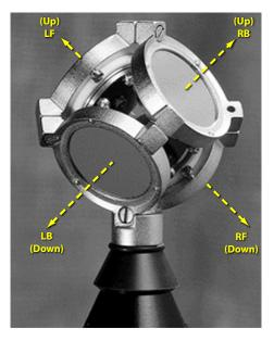
Figure 3.9 Four-capsule microphone positioned in a tetrahedron. The soundfield can be defined by an omnidirectional pressure and three difference pressures in X, Y, Z direction(©Soundfield).
