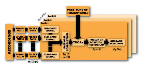
Figure 6.3 Overview of the analysis algorithm used to construct a spatial mapping for the acquired soundscapes.
