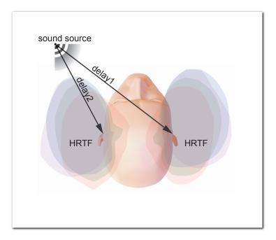
Figure 4.3 Audio processing involved in the GPU simulation. Each sound source is delayed by the propagation time and filtered to account for the distance attenuation and head-related transfer functions (HRTFs).
