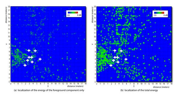
Figure 7.3 Comparison between energy localization in the seashore example of Section 7.3 for (a) the foreground component only and (b) the complete recording. The figure shows the reconstructed location of all subbands integrated through the entire duration of the sequence. White crosses indicate the locations of the microphones used for recording.
