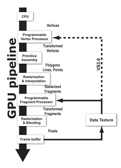
Figure 4.1 GPU pipeline. The vertex processor and the fragment processor are totally programmable.
