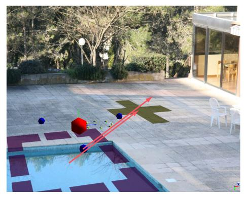
Figure 6.15 An example interface for source re-localization. In this example we select the area corresponding to the fountain (in purple) and translate it to a new location (shown as a yellow cross). The listener is depicted as a large red sphere, the microphone array as small yellow spheres and the blue spheres show cluster locations.
