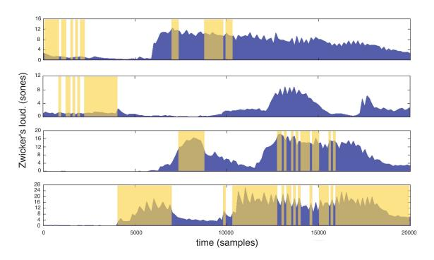
**Figure 5.1** Four speech signals prioritized according to a loudness metric computed over successive short time-frames. The single most important frame across time is highlighted in yellow.
