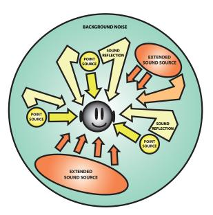
**Figure 7.1** Typical components of a real-world auditory scene. In this chapter, we propose to explicitly separate *foreground*, non-stationary and well localized, sound events from *background* components that are more stationary and spatially diffuse.
