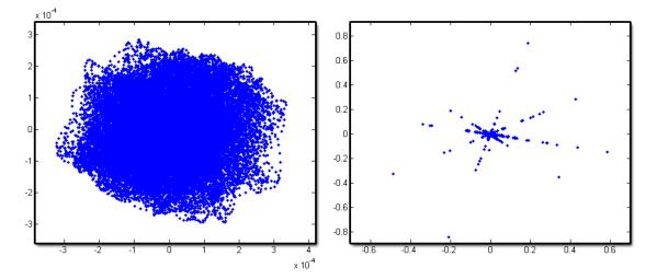
**Figure 3.1** Data sparseness : (a) Scatterplot of two linear mixtures in the time domain. (b) Scatterplot of two linear mixtures in the frequency domain. Note : In the frequency domain, lines appear and their directions correspond to the mixing coefficients used for the mixture.
