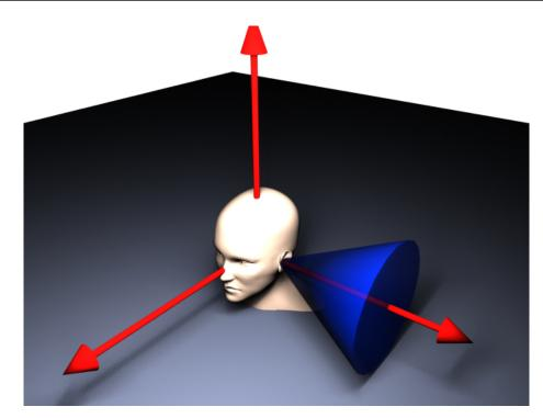
Figure 2.11 The cone of confusion : Different spatial locations produced null ITD and ILD in this area.
