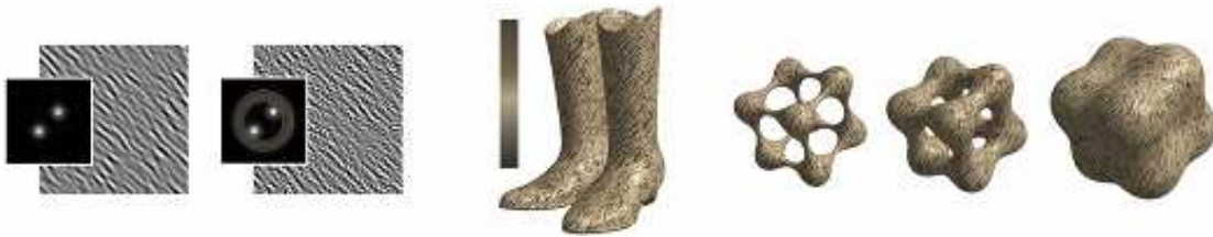
Figure 1: Modeling the appearance of objects with noise. (Left) A noise pattern is designed by a user. (Middle) A leather texture is obtained by combining the noise pattern with a color map. (Right) The leather texture is mapped onto a dynamically changing implicit surface. (Figure from [LLDD09].)
