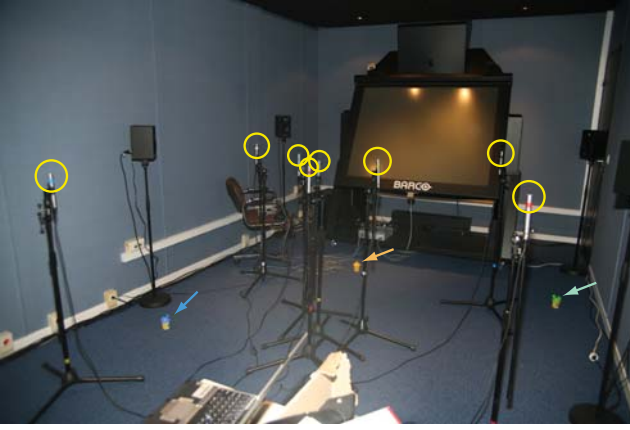
Figure 7: Indoor validation setup using 8 microphones. The 3 markers (see blue, yellow, green arrows) on the ground correspond to the location of the recorded speech signals.
