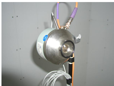
Figure 6: Our reference source, the Brüel&Kjaer artificial mouth .
