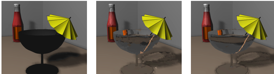
Fig. 6. A radiosity solution (left) is corrected towards a ray tracing solution using 5,000 (0.48 %), and 20,000 (1.9 %) ray tracing samples (center and right).
