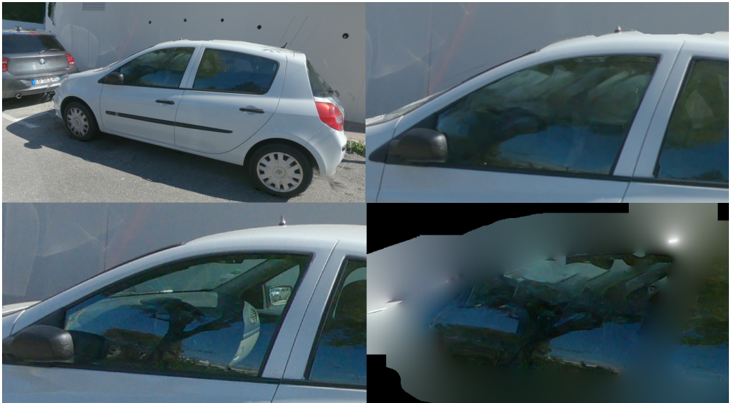
Fig. 3. Top left: novel view rendering with our method. Top right: crop of the view; rendering artifacts are visible. Lower left: closest input view; there is a strong discontinuity on a bright background with some reflections present. Lower right: reflection layer min-composite in this case.
