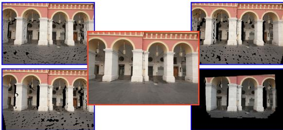
Figure 5: The four side images show the warped superpixels of 4 input images pre-selected to render the current novel view. The central image shows the blended result of the 4 warped images.
