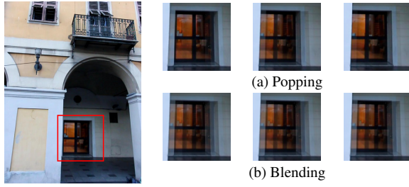
Figure 1: Transitional artifacts visible in 3 consecutive frames (25 fps) on the door under the arch. (a) Popping, with some visible blending in the middle frame. (b) Mixing 3 input images.
