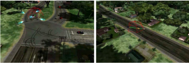
Figure 4: Sound source clustering in the Test Drive Unlimited engine. Red wireframe spheres are clusters. ©Eden Games-ATARI 2006.
