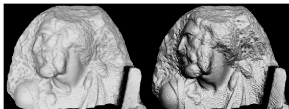
Figure 7: Upper part of the St Matthew model with our method rendered at 165 FPS, without (left) and with (right) the normal maps. The maps are recreated directly from the point cloud, providing a convincing appearance, while using less than 80k triangles (left image). Most of the “appearance” information carried by the original point cloud is directly stored through these normal textures on the GPU memory (185 MB) and used for the per-pixel lighting.
