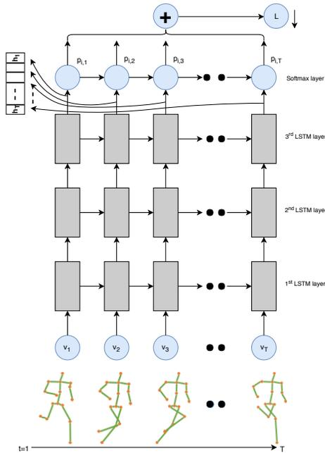
Figure 1. Three-layer stacked LSTM with  $t = T$  time steps. The skeleton joint coordinates  $v_t$  are input at each time step.  $L$  is the loss computed over time and  $h$  is the latent vector from last layer LSTM which is input to the linear SVM classifier.
