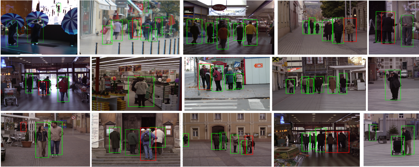
Fig. 5. Detection examples on the INRIA dataset. Green boxes represent our algorithm detections, the brightness being set in relation to their confidence. Red boxes depict missed detections. Best viewed in color.
