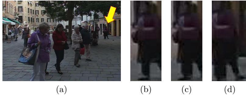
Figure 1: An example of the re-ID (Fast-reid [5]) being confused. At frame t (a), the bounding box of the considered person (b) was associated with the bounding box of the other person (d) at t-1 instead of the same person (c) at t-1 . Match was based on the minimum re-ID cosine distance score. Such cases might pose difficulties also to human observers. Source: MOT17 [11].
