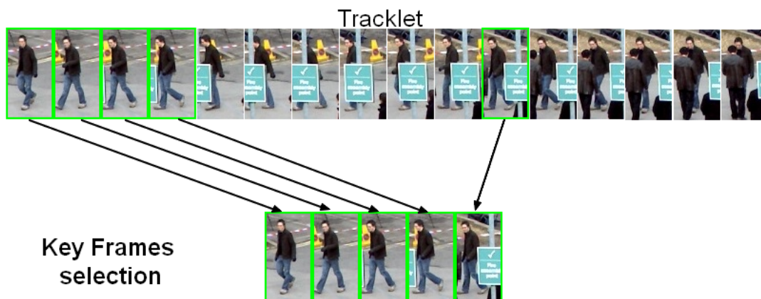
Figure 3.2: Selection of the most reliable nodes to be used as key frames
