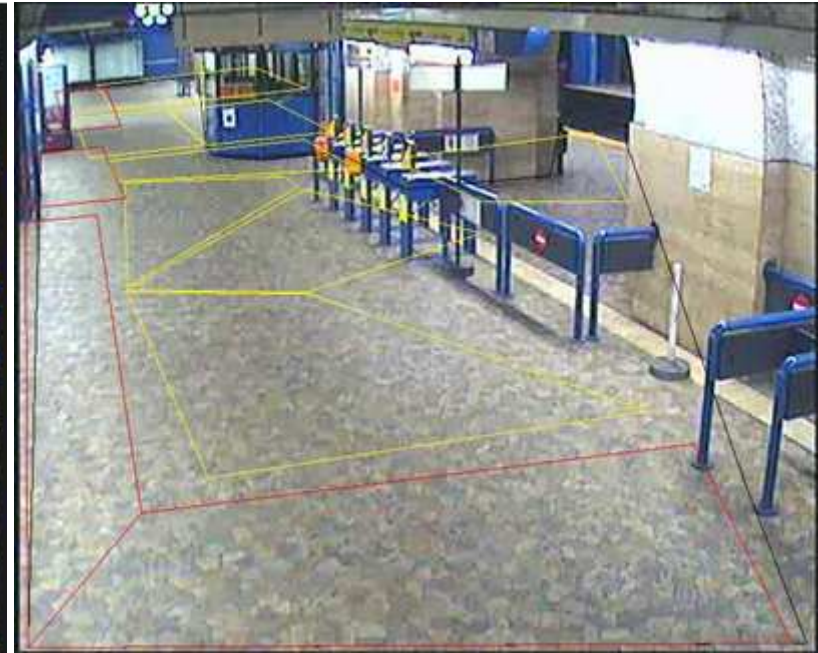
The yellow polygons show the outline of the learned lost zones. The red polygons show the outline of the entry zones, exit zones.
