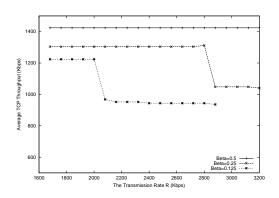
Figure 4: Simulation: TCP throughput vs. R
