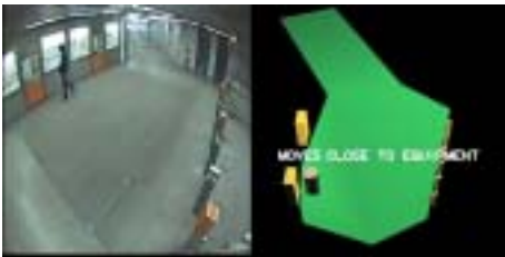
Figure 7. After a short period, the person comes back to the ticket machine: A fact event named moves close to equipment is created
