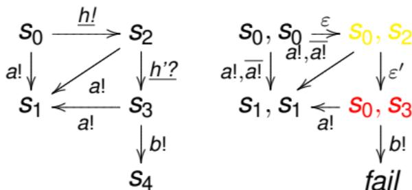
In this case, if we remove transition  $s_2 \xrightarrow{h'?) s_3}$ , we obtain a secure interface:
