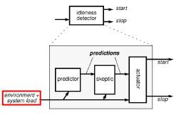
Proposed Model for Idleness Detection Metric Collection Predicting Values Adjusting Predictions Integration with ProActive's P2P
