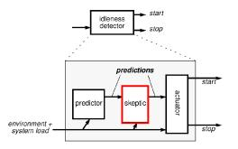
Proposed Model for Idleness Detection Metric Collection Predicting Values Adjusting Predictions Integration with ProActive's P2P
