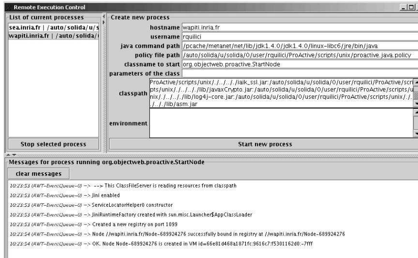
Fig. 9. Interactive creation of a new JVM and associated node
