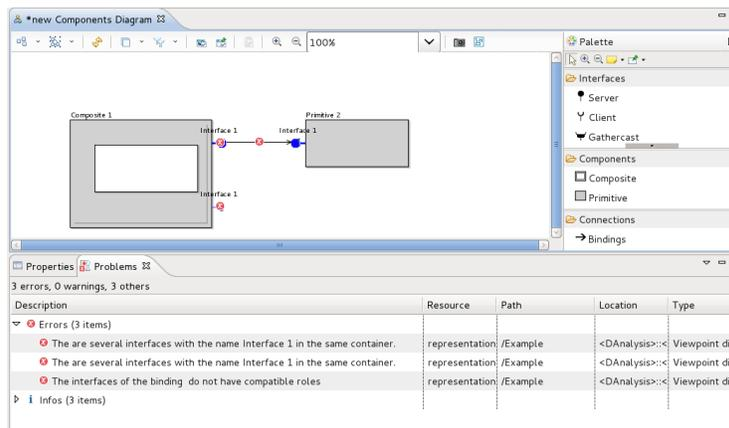
The interfaces of Composite1 did not pass the validation because they have the same names. The binding did not pass the validation because it goes from a server interface to a server interface.
