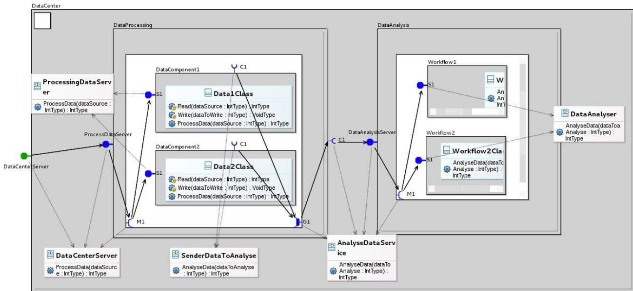
This is a typical High performance component architecture, where the work is dispatched on groups of components (e.g. {DataComponent 1,2}) through a multicast interface M1.
