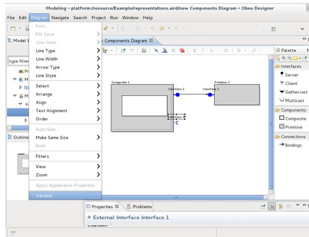
The elements of the diagram which did not pass the validation should be marked with red signs. You will also see the validation errors/warnings description in the “**Problems**” tab, and in the Model explorer.
