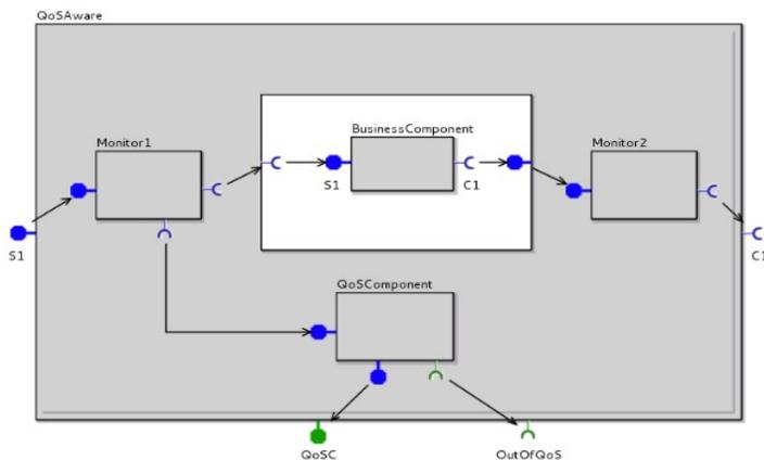
This is an example demonstrating the use of non-functional components in the membrane, for monitoring the quality
