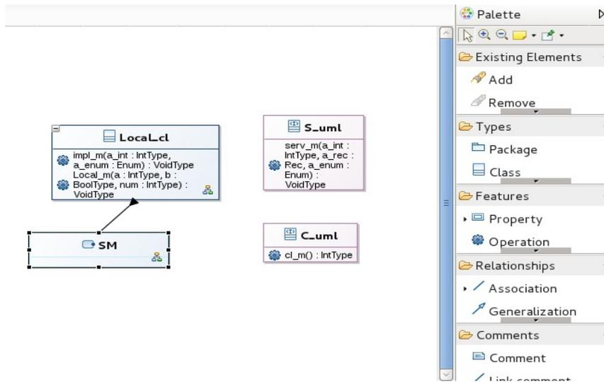
It has two UML Interfaces: **S\_umI** and **C\_umI**, and one UML Class **LocalCl**. In order to create them, “**Interface**” (resp. “**Class**”) tools are used.
