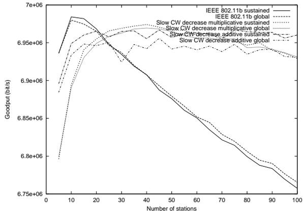
Figure 8: Simulation of the obtained rates with the RTS/CTS mechanism.
