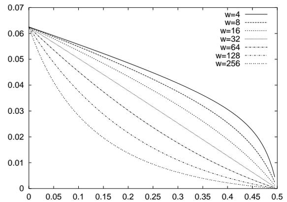
Figure 6: Different access probabilities for  $W_0 = 32$ ,  $p_c = p$ , and  $q = 1 - p$ .
