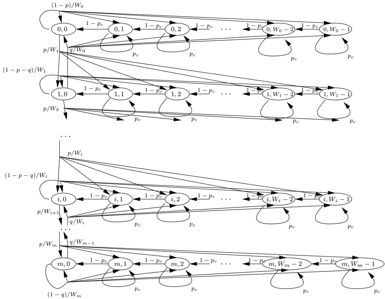
Figure 4: The Markov chain for the additive model.
