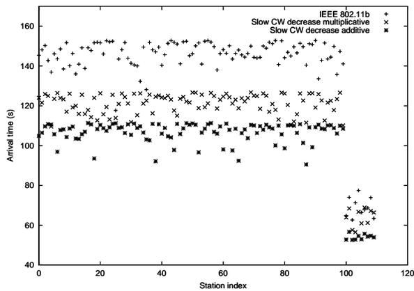
Figure 9: Completion times for the stations with the basic mechanism.
