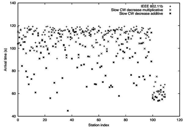
Figure 10: Completion times for the stations with the RTS/CTS mechanism.
