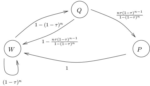
Figure 3: General figure of the slotted CSMA/CA process.
