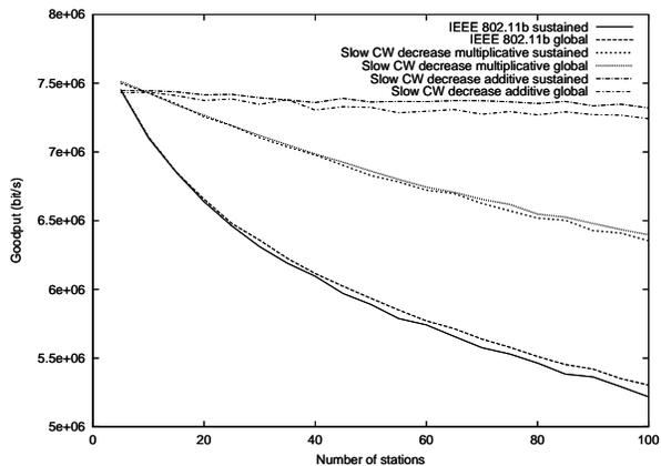
Figure 7: Simulation of the obtained rates with the basic mechanism.
