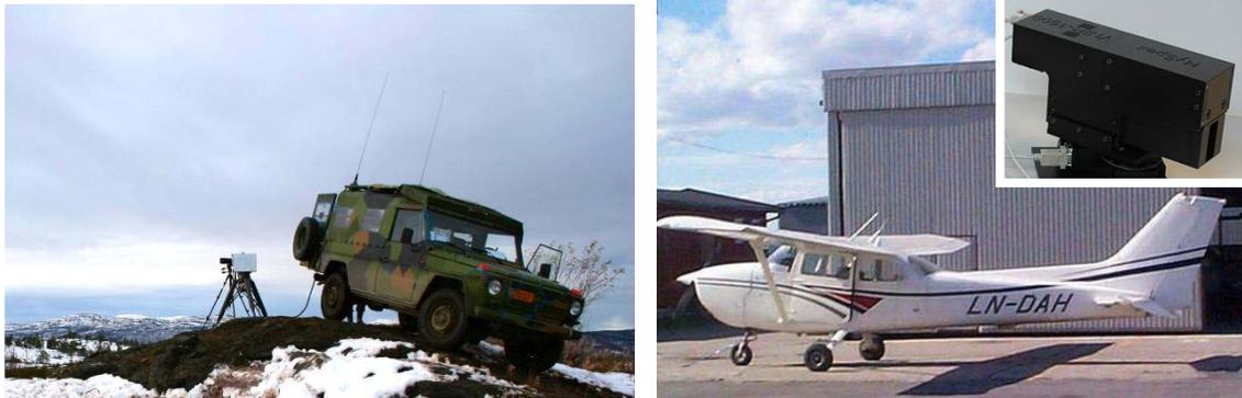
**Figure 2. A ground-based camera setup has been built for operational testing in ground-to-ground scenarios. The picture on the left shows an early trial of the ground based system in northern Norway. On the right is the Cessna 172 which has now been modified to accommodate the airborne demonstrator system. The inset shows the HySpex VNIR hyperspectral camera to be fitted in the aircraft together with a real-time processing system and supplemental sensors.**
