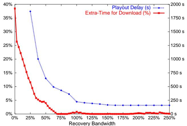
Figure 5 Rome-Florence railways path: Delayed Real-Time zero-loss trade-offs (right y-axis) and Multimedia-on-demand performance (left axis)
