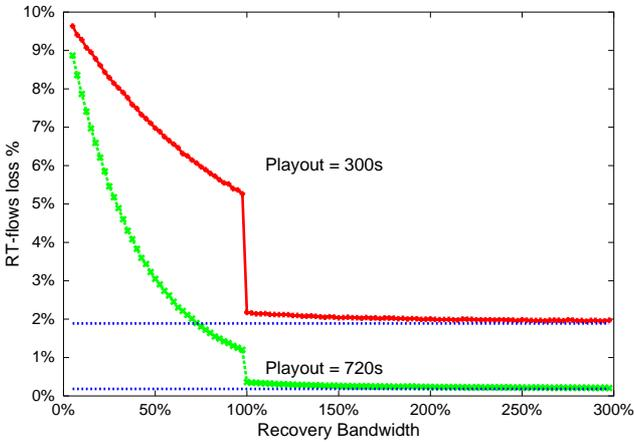
Figure 4 Delayed Real Time stream: fraction of unrecovered (lost) data
