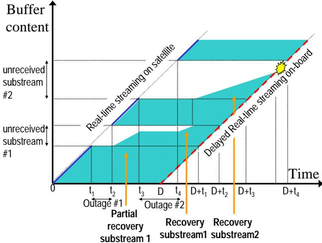
Figure 2 Real-Time Connection outage after multiple channel outages
