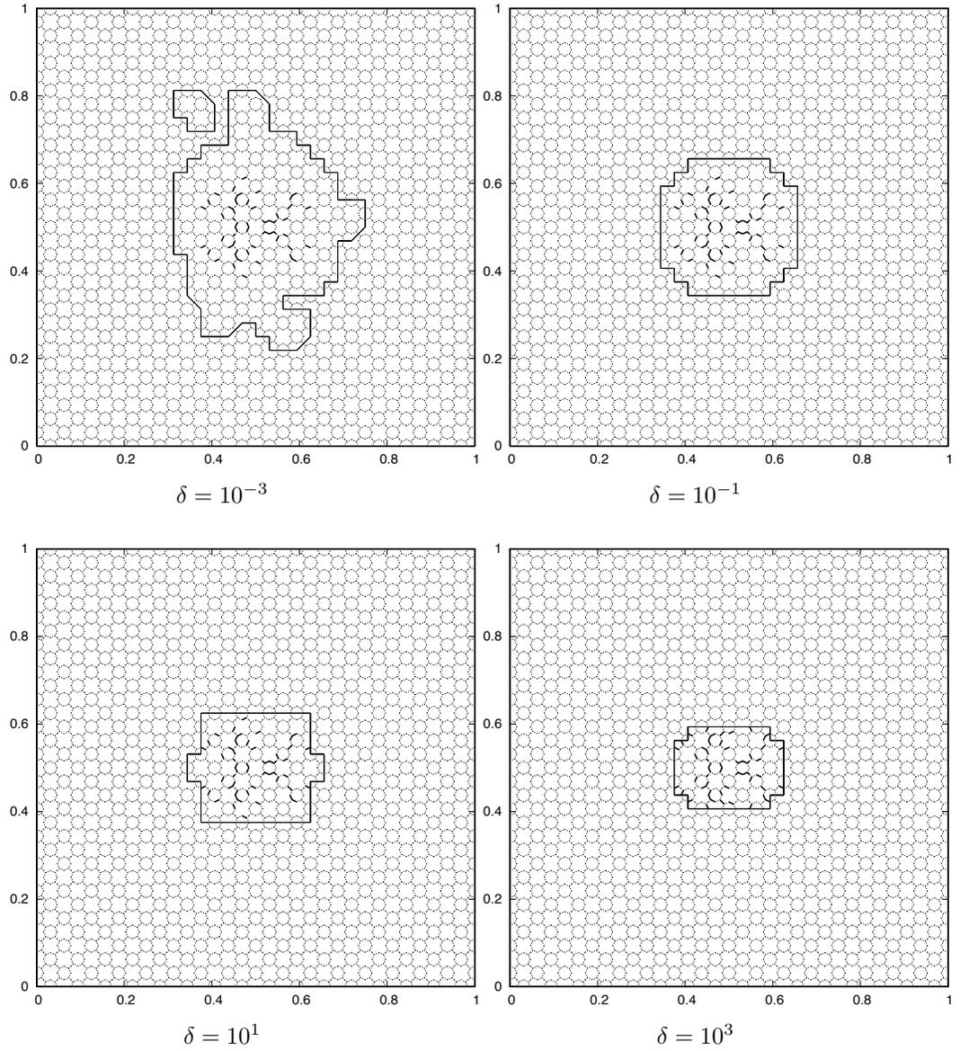
Figure 10: Product  $\langle Q_f; \nabla_t \theta \rangle$  defined by (4.5) and sub-domains interface for several value of  $\delta$ . Dotted lines are faces with product  $\langle Q_f; \nabla_t \theta \rangle$  negative, thick plain lines are faces with product  $\langle Q_f; \nabla_t \theta \rangle$  positive and thin plain lines are sub-domains interface.
