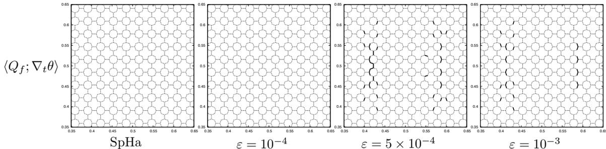
Figure 7: Product  $\langle Q_f; \nabla_t \theta \rangle$  defined by (4.5) with (2.11) (first figure) and with (2.15)-(2.16) for several value of  $\varepsilon$  (second and fourth figure) zoomed on the central area at  $t = 5h_t$ . Dotted lines are faces with  $\langle Q_f; \nabla_t \theta \rangle \leq 0$  and full lines are faces with  $\langle Q_f; \nabla_t \theta \rangle > 0$ .
