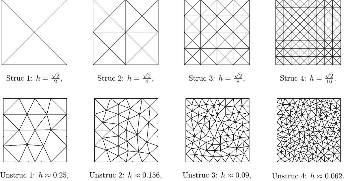
Figure 3: Examples of mesh used to estimate the consistence. In the first line, structured meshes obtained with iterative process, Struc  $n$  is the union of four Struc  $n - 1$  scaled by  $1/2$ . In the second line, unstructured meshes obtained by Delaunay triangulation using the mesh generator *Triangle*.
