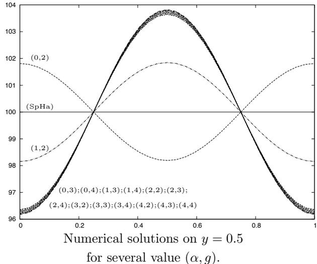
Figure 5: Numerical results for several value of  $(\alpha, g)$ . The left tabular is the  $L^\infty$  norm of the solution. The right figure is the temperature profile on the hyperplan  $x_2 = 0.5$ .
