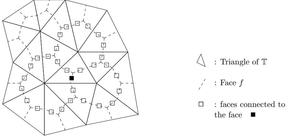
Figure 1: Example of control volume  $\mathcal{C}_k$  and connectivity.
