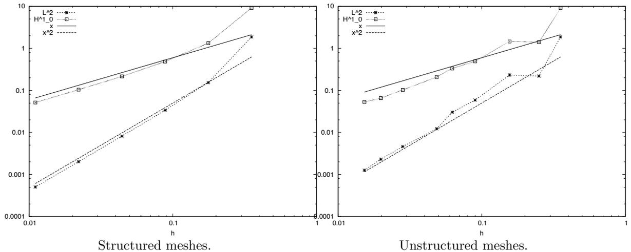
Figure 4: Errors in the  $L^2$  norm and in the  $H_0^1$  norm between the numerical and the analytical results.
