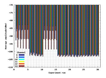
Fig. 5. Average signal power per channel per run in test cases [1,6]
