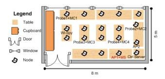
Fig. 1. Wireless testbed setup and placement of nodes
