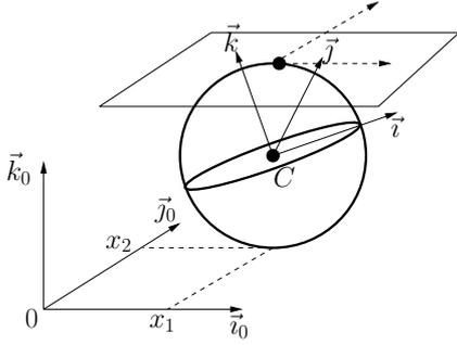
Fig. 1. The rolling sphere actuated by a moving plate
