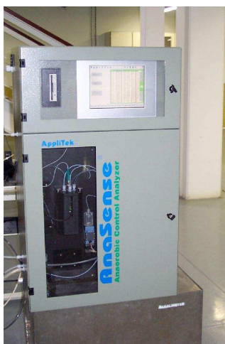
Figure 2. Validation of the AnaSense sensor dedicated to the measurement of VFA, bicarbonate, total and partial alkalinity.
