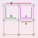
$\begin{array}{l} \mbox{Request } d: 1 \rightarrow 3 \\ \mbox{Request } e: 6 \rightarrow 5 \\ \mbox{Request } c: 2 \rightarrow 3 \\ \mbox{Request } b: 1 \rightarrow 5 \\ \mbox{New link } \{8,9\} \end{array}$
