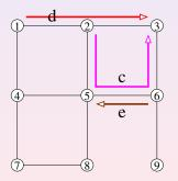
$\begin{array}{l} \mbox{Request } d \ : \ 1 \rightarrow 3 \\ \mbox{Request } e \ : \ 6 \rightarrow 5 \\ \mbox{Request } c \ : \ 2 \rightarrow 3 \\ \mbox{Rerouting of request } e \end{array}$
