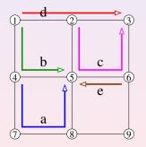
$\begin{array}{l} \mbox{Request } d : 1 \rightarrow 3 \\ \mbox{Request } e : 6 \rightarrow 5 \\ \mbox{Request } c : 2 \rightarrow 3 \\ \mbox{Request } b : 1 \rightarrow 5 \\ \mbox{Request } a : 4 \rightarrow 5 \end{array}$
