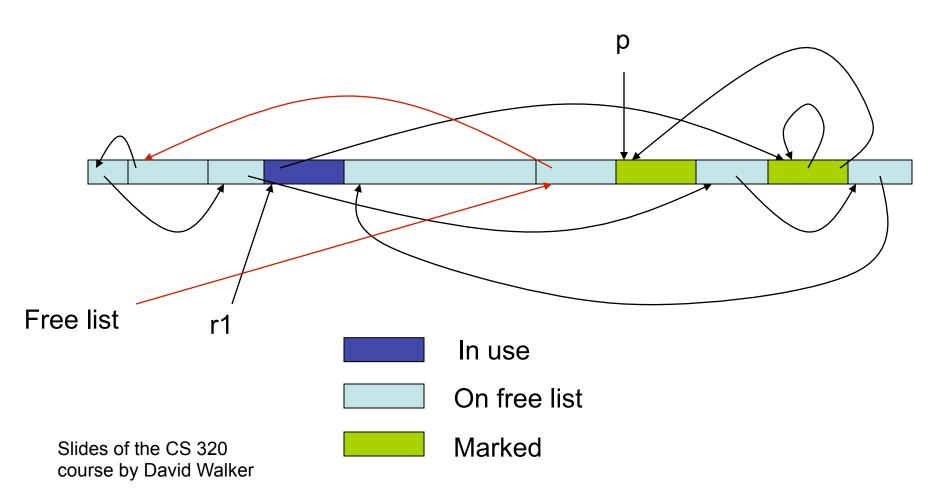
Sweep Phase: GC complete when heap boundary encountered; resume program
