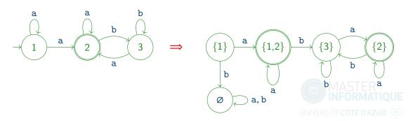
A deterministic finite automata (DFA)  $\mathcal{A}$  is a NFA where each state has precisely one successor state:
