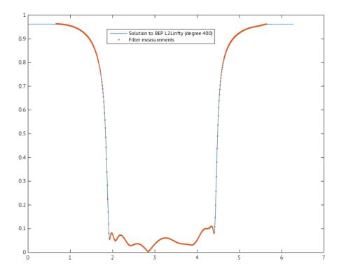
Figure 1: Solution of DBEP at hand of partial scattering measurements of a microwave filter
