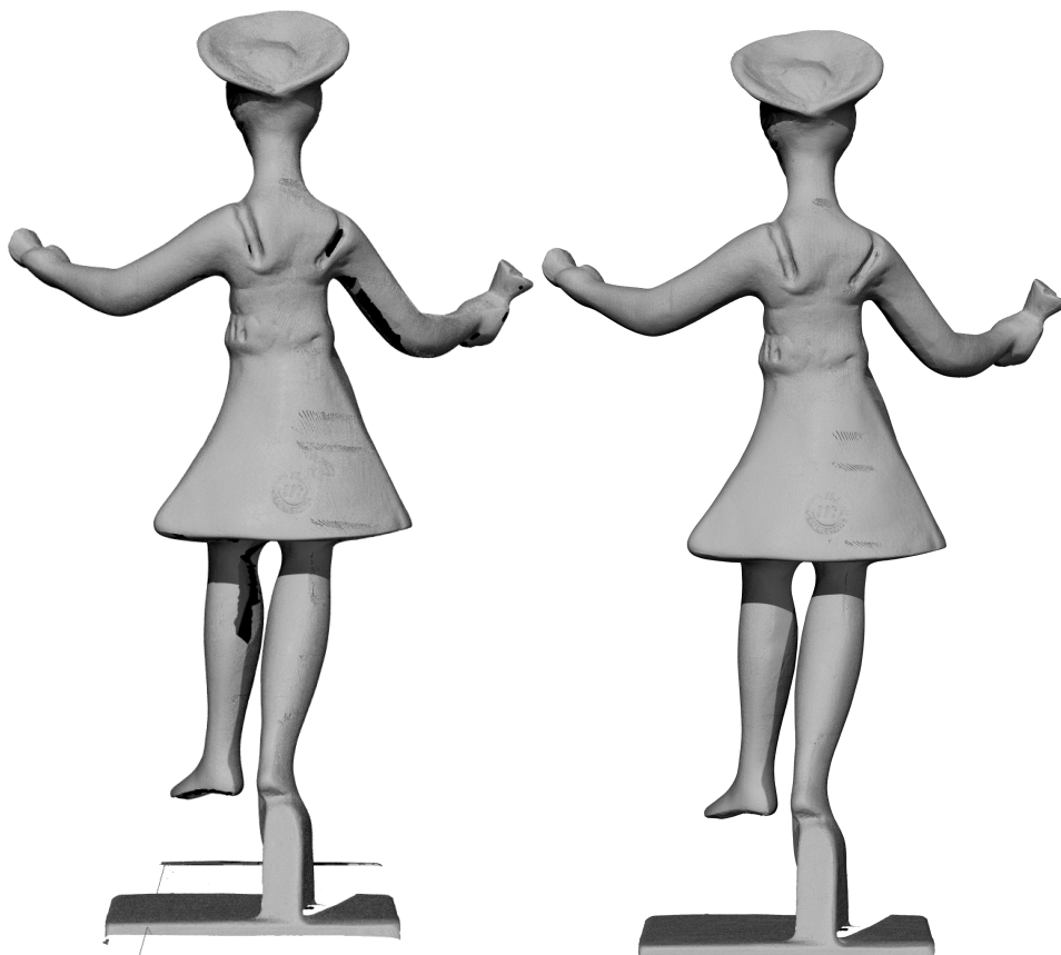
Figure 5.6: Dancer with Crotales: fine scale mesh (left), fine scale mesh with filled holes (right) , here the base hole patch is removed
