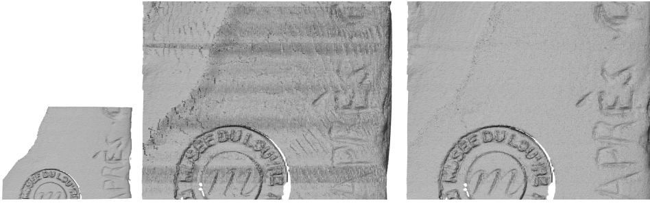
Figure 4.11: Comparison of a rendering of a single scan (ground truth) and the merging of all scans that overlap in the same region (Left: ground truth, middle: joint mesh of all scans without merging, right: joint mesh with merging).
